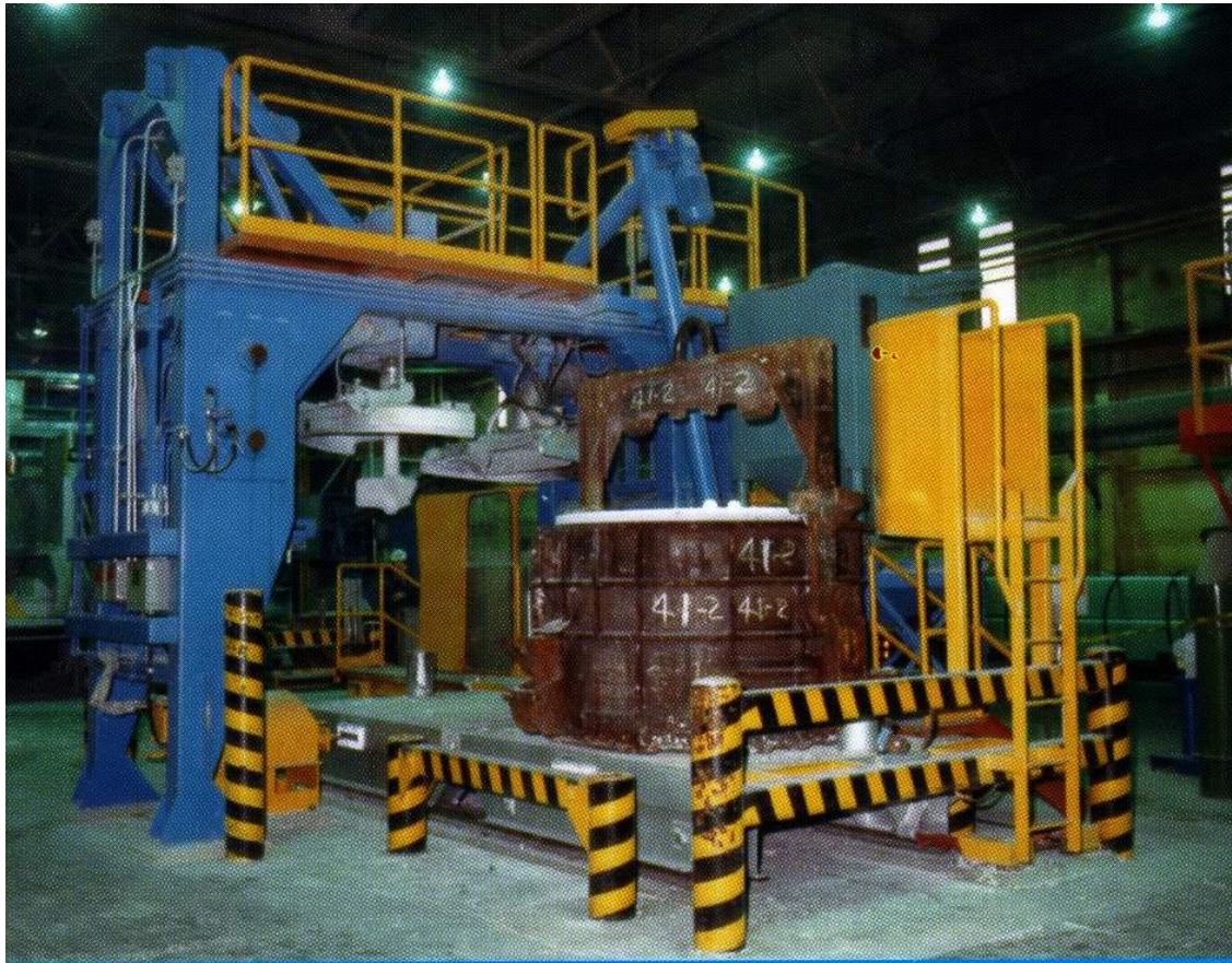
AUTOMATED TAC TREATMENT STATION, ONE CRUCIBLE (ON THE RIGHT) BEING TREATED, THE OTHER CRUCIBLE IS READY FOR TREATMENT
